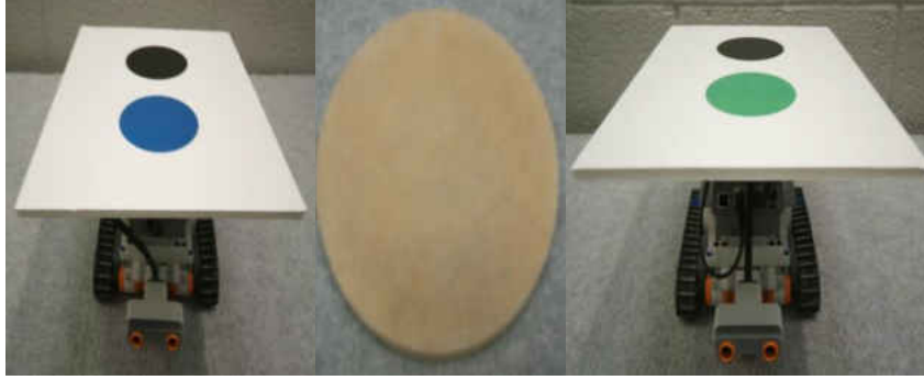
Figure 24: Vision system identifiers used by robots (left and right) and example obstacle (middle).
