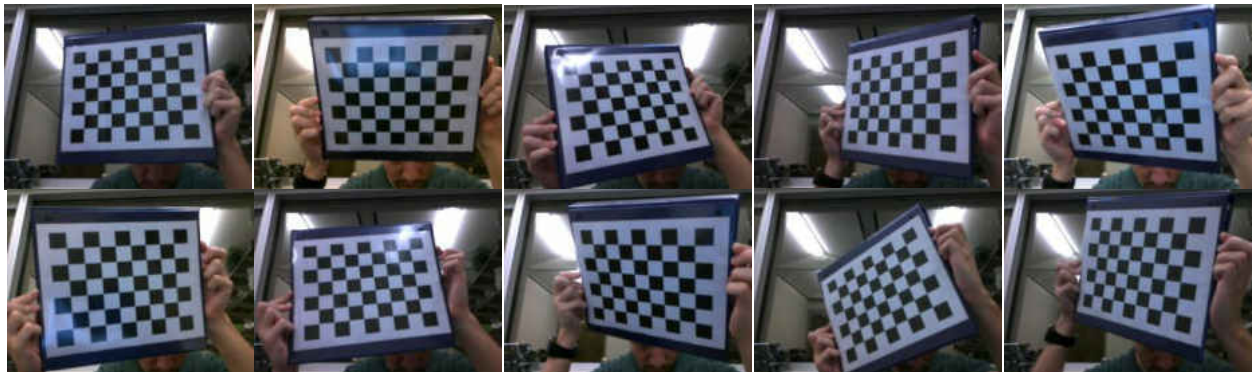
Figure 3: Example of images used in calibration.
