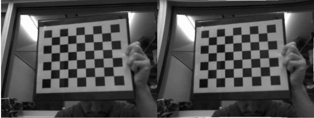
Figure 4: Image from camera before (left) and after (right) distortion calibration
