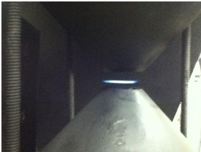
Figure 8 - First successful ignition of counter-flow flame in this work
