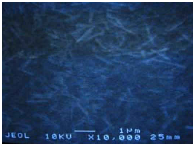
Figure 5 SEM picture of Cu/CNT composites Composites is fabricated by the electrochemical co-deposition[147]
