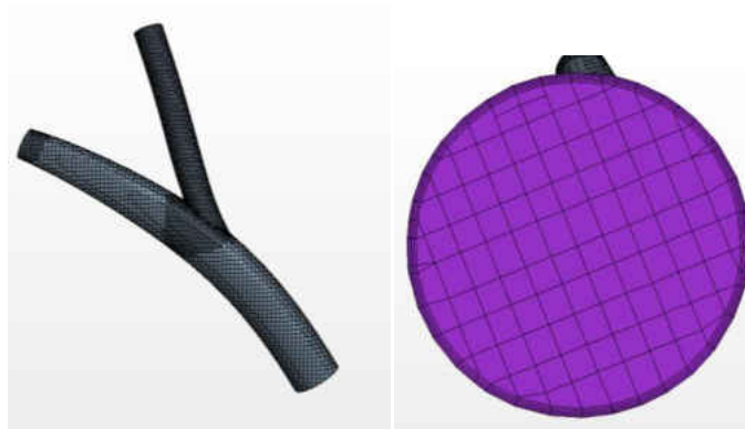
Figure 7: Bifurcation fluid mesh
