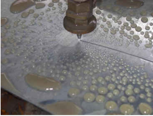
Figure 2: A high pressure jet is cutting aluminum sheet (Eggers and Villermaux, 2008)
