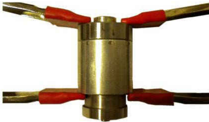
Figure 13: Completely Assembled Magnetic Bearing Forced into Alignment
