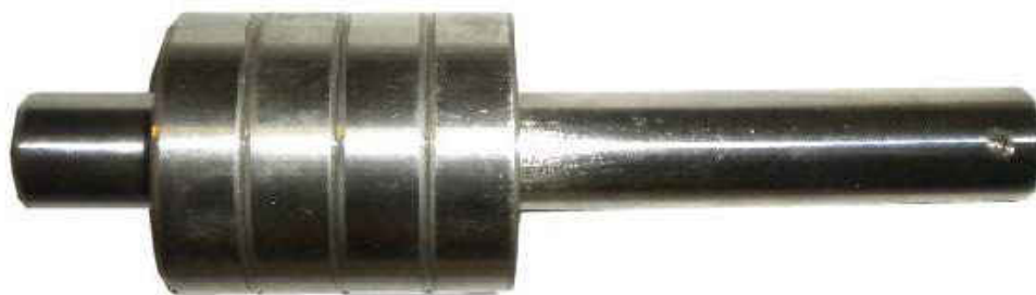
Figure 19: Reference Ball Bearing Shaft Configuration
