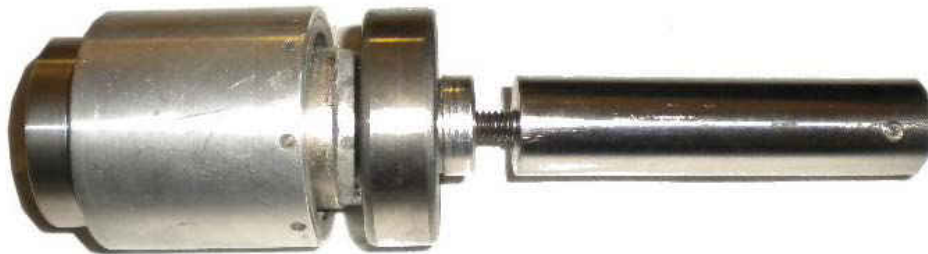
Figure 18: Magnetic and Ball Bearing Shaft/Coupler Configuration
