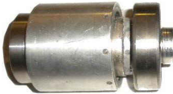
Figure 12: Completely Assembled Magnetic Bearing in Shifted Position
