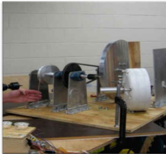
Figure 9: First alternative laboratory prototype using pulley and cable
