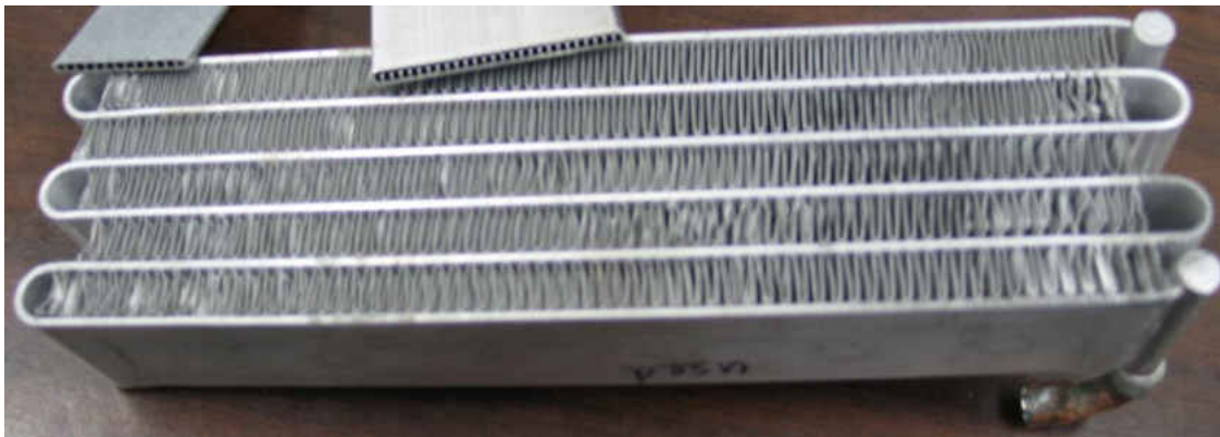
Figure 22. Picture of the traditional air-cooled condenser
