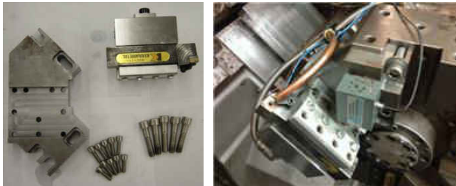
Figure 3-6: (Left) Dynamometer assembly (Right) Dynamometer mounted on lathe
