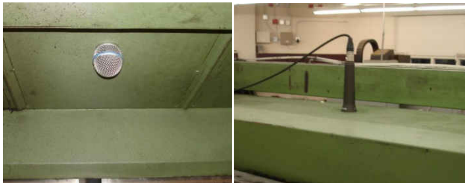
Figure 3-11: (Left) Interior view of microphone (Right) Exterior view of microphone
