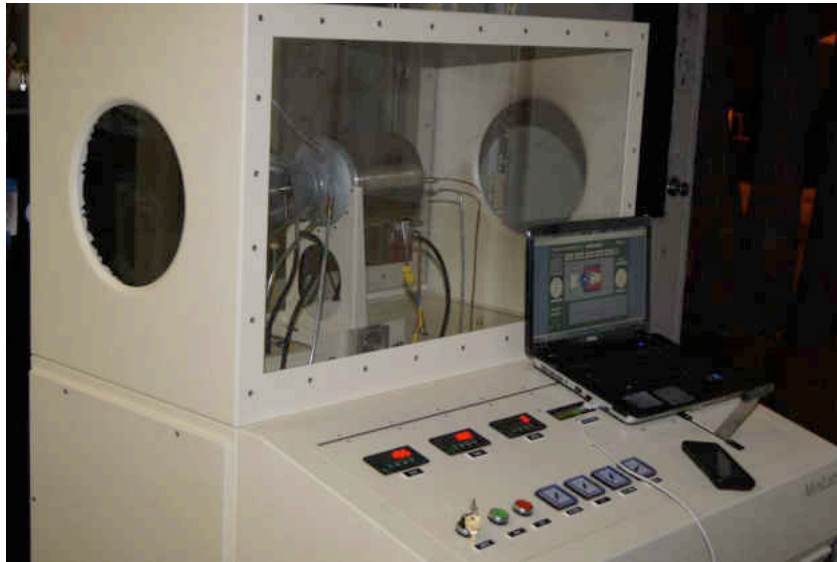
Figure 5 – Photograph of SR-30 engine used in testing
