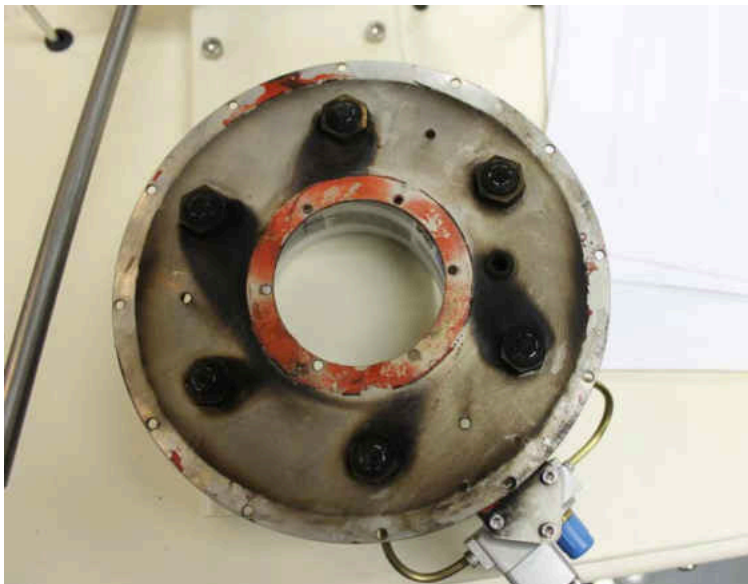
Figure 21 – SR-30 Engine fuel injectors before overhaul
