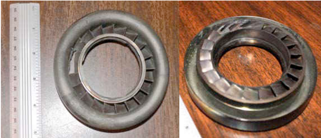
Figure 18 – Turbine stator damage
