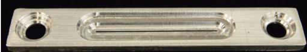
Figure 10: Extractor machined in aluminum with a 0.5mm slot
