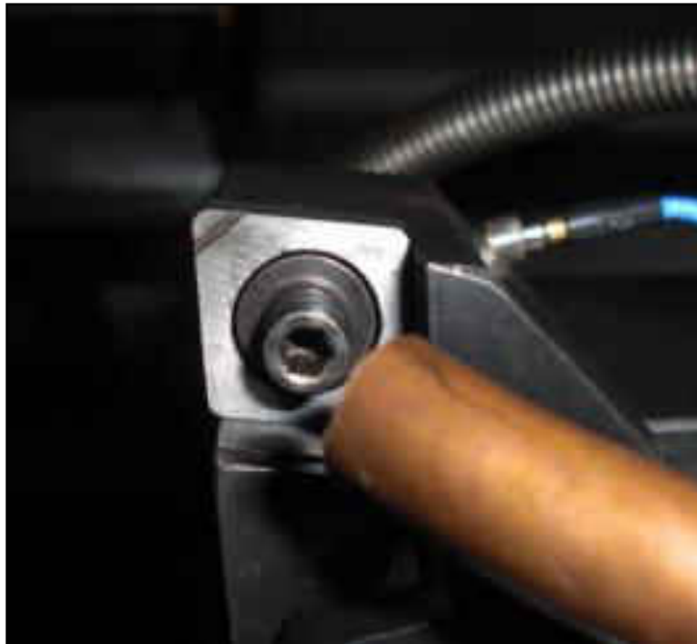
Figure 15: Groove Location for Thermocouple on Insert
