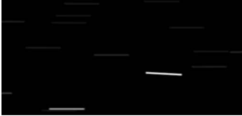
Figure 4.1: Sample star camera image containing and RSO with apparent motion.
