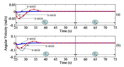
Figure 8: Angular Velocities of the Satellites in the 1<sup>st</sup> Attitude Control Period: a) Satellite One; b) Satellite Two
