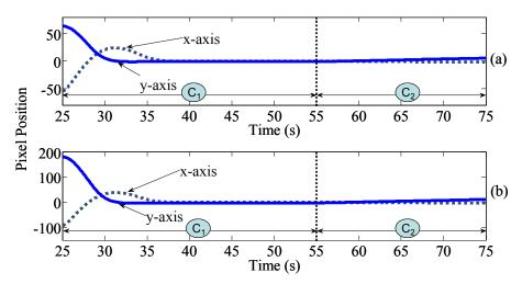
Figure 14: The Pixel Locations of the Debris in the 1<sup>st</sup> Attitude Control Period: a) Satellite One; b) Satellite Two
