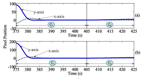
Figure 15: The Pixel Positions of the Debris in the 2<sup>nd</sup> Attitude Control Period: a) Satellite One; b) Satellite Two
