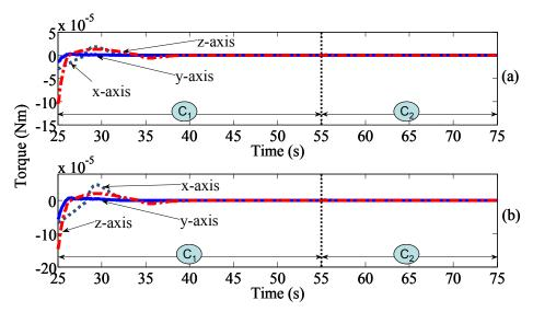
Figure 12: Torque Commands During the 1<sup>st</sup> Attitude Control Period: a) Satellite One; b) Satellite Two
