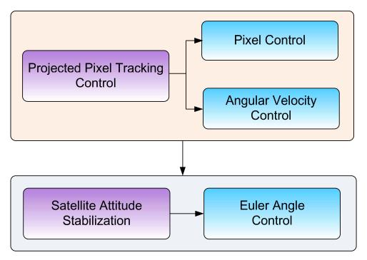
Figure 4: Overall structure of attitude control
