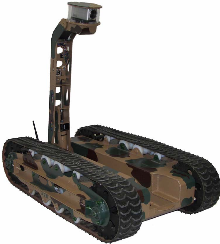
Figure 4 : The tread driven all-terrain autonomous surveillance robot
