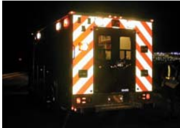
Figure 3: Chevron Pattern at night – Reflectors
