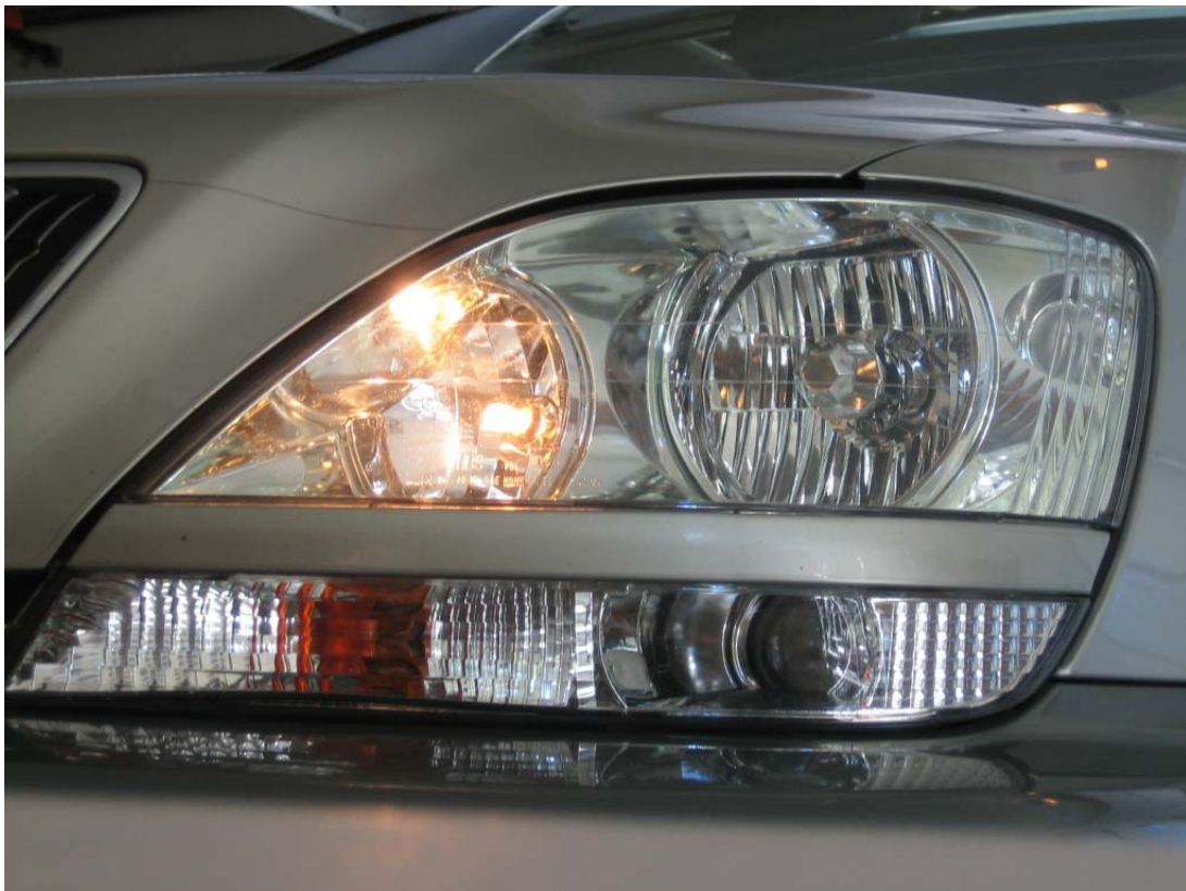
Dedicated DRLs (separate light within headlight housing)
