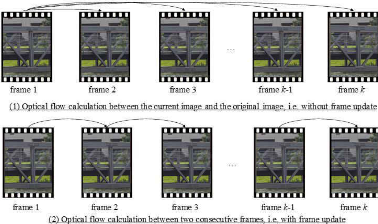
Figure 43 Two different strategies to process image sequences and get displacement time histories
