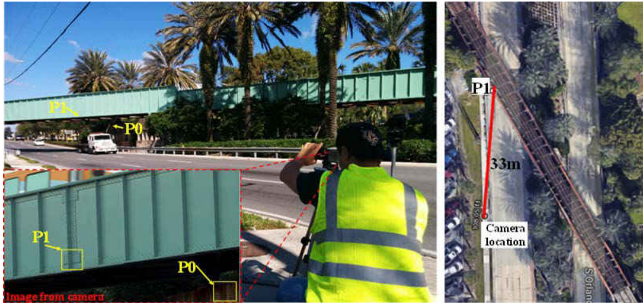
Figure 35 Experimental setup for a railway bridge
