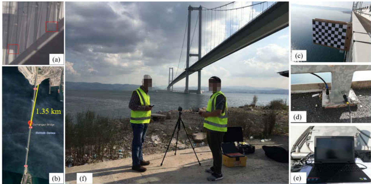
Figure 81 Experimental setup of the first experiment of the Osman Gazi Bridge: (a) image from camera, (b) camera location in map; (c) wood chessboard, (d) accelerometers in vertical and horizontal direction, (e) computer for data acquisition, (f) camera setup
