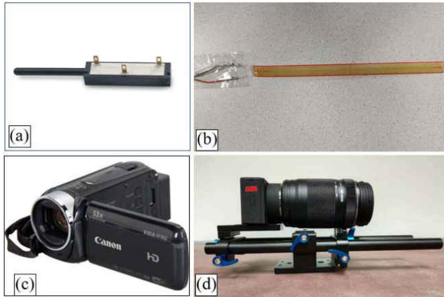
Figure 104 Sensors and cameras used in the test: (a) displacement sensor, (b) strain gauge, (c) camera for traffic monitoring, and (d) camera for displacement measurement
