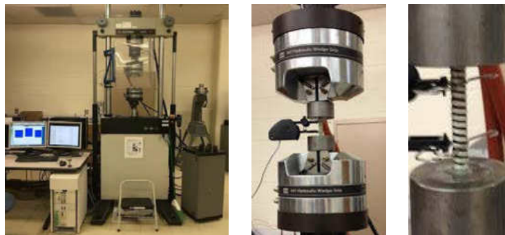
Figure 2.8: Instron Test Machine: Full Instron Test Machine (top left); Extensometer Attached to Specimen (center); and, Specimen Being Held by Test Specimen Receptacles (right)
