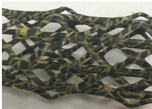
Figure 1.1 Example of a Typical IsoTruss Structure
