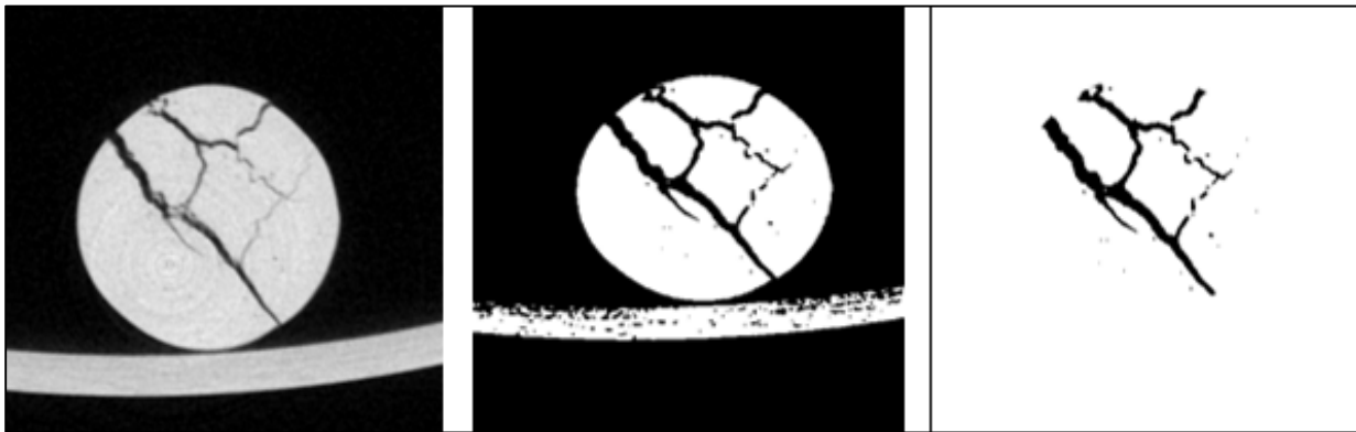
Figure 2.7 Procedure for Quantifying Damage based on Micro-CT Scans: Initial Image (left); Binary Image (center); and, Crack Area (right)
