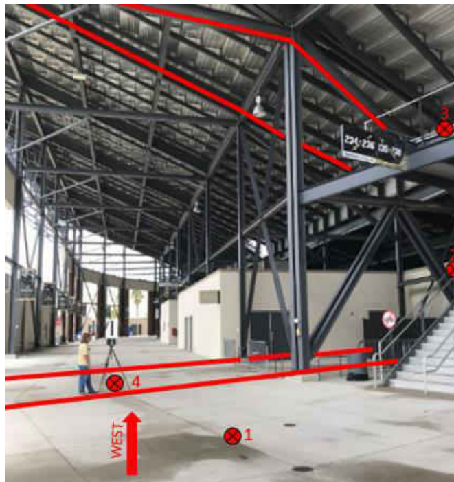
Figure 3.7: Limits of scan area shown by red lines. Marks 1-4 indicate the four scanning locations. Source: Sofia Baptista and Jacob Solomon
