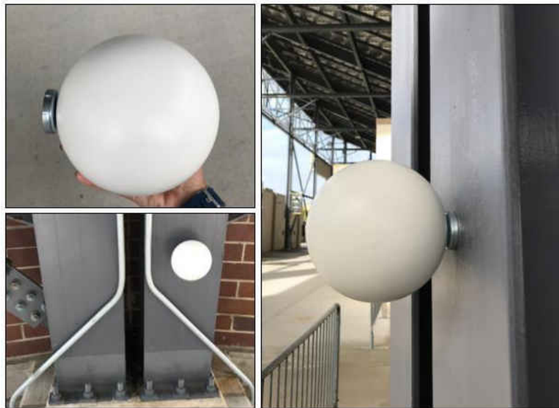
Figure 3.5: Tracking balls used on-site Source: Sofia Baptista and Jacob Solomon
