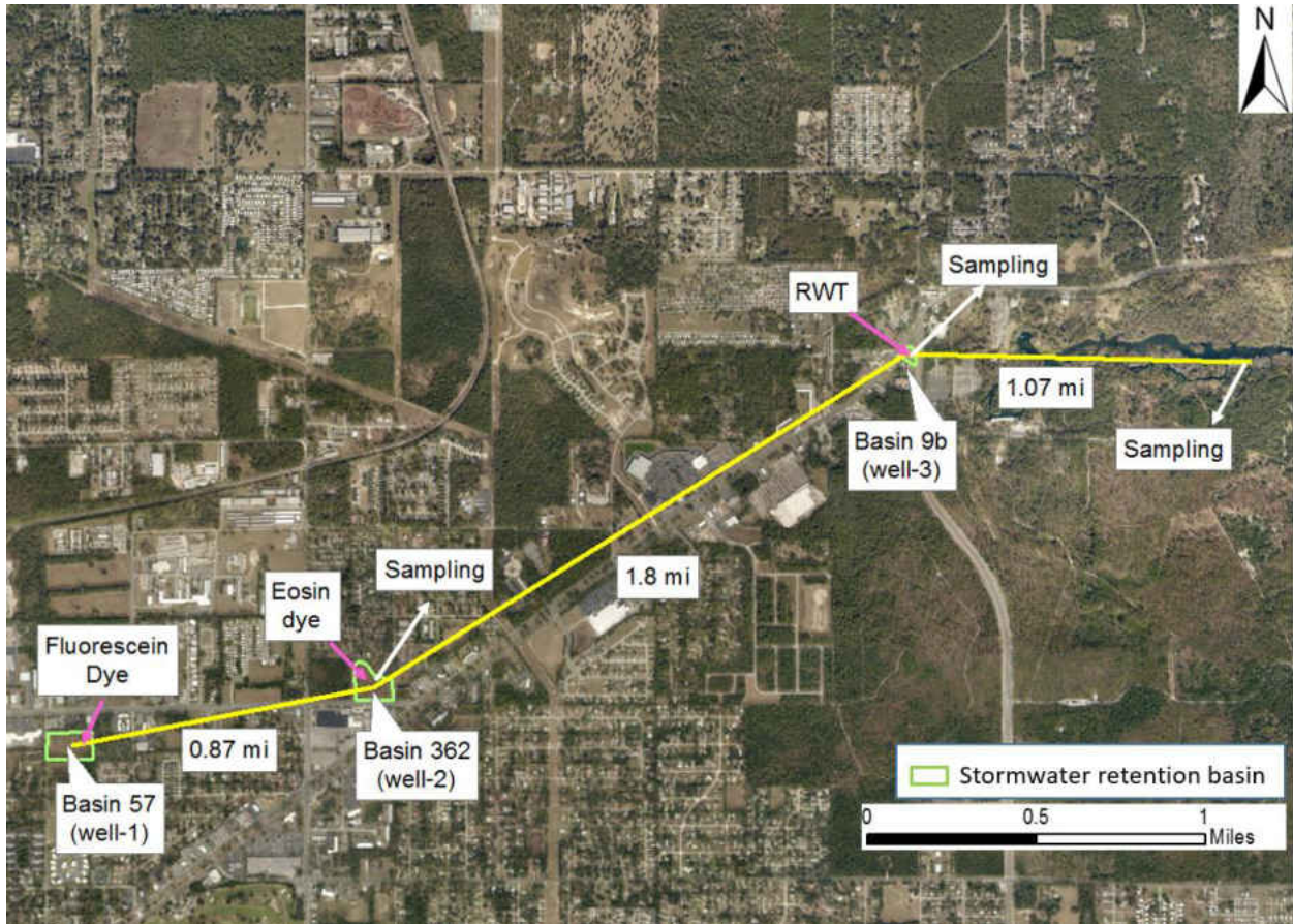
Figure 7: Injection and sampling sites for the tracer dyes.
