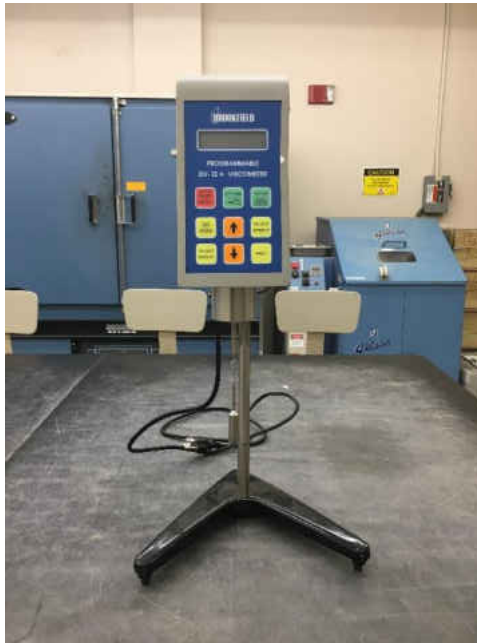
Figure 4-2. Viscometer device used to measure the viscosity of cement pastes
