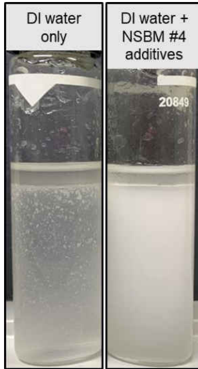
Figure I. 1. Emulsion formation using pure DI water and DI water exposed for 24 hrs to NSBM #4. Bulk-water was emulsified with 10% v/v mineral oil.
