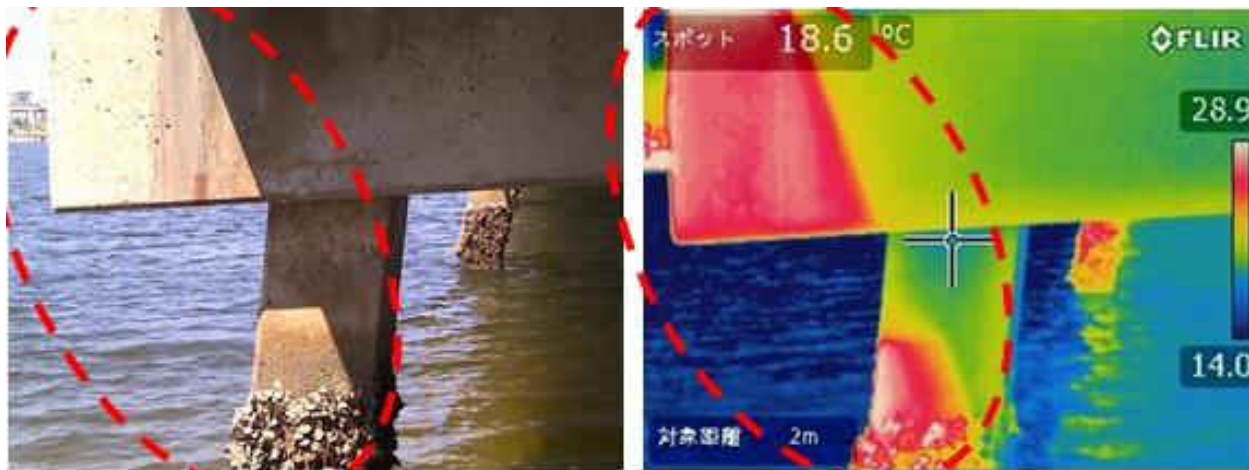
Figure 21: Effect of solar radiation on IRT detection result
