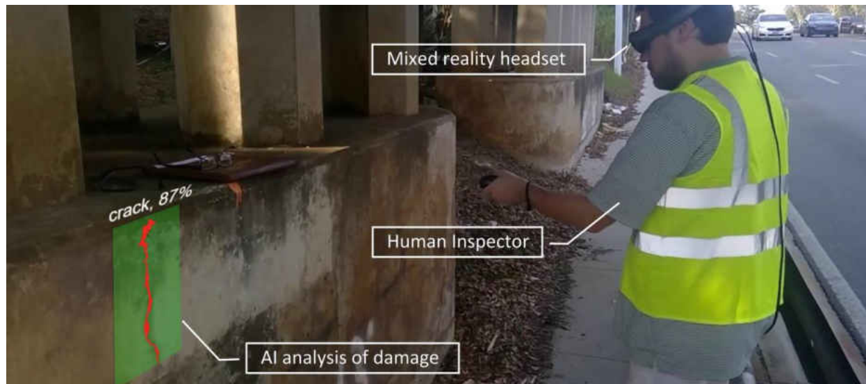
Figure 30: Visual representation of the AI powered mixed reality system. (The headset user interface and analysis environment are shown for illustration purposes.)
