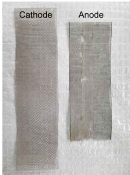
Figure 5-6: Electrodes used in the EFO system: Running under low and high intensities for about 10 days; The anode releases stainless steel particles due to electrolysis.
