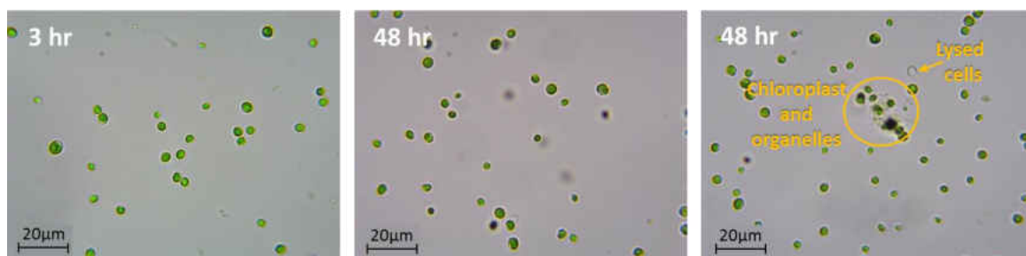
(d) Applied potential: -0.4 V; conductivity: 4630.9 \mu\text{S cm}^{-1} , Electrode type: Stainless steel mesh.
