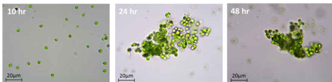
(c) Applied potential: -0.1 V; conductivity: 4630.9 \mu\text{S cm}^{-1} , Electrode type: Stainless steel mesh.
