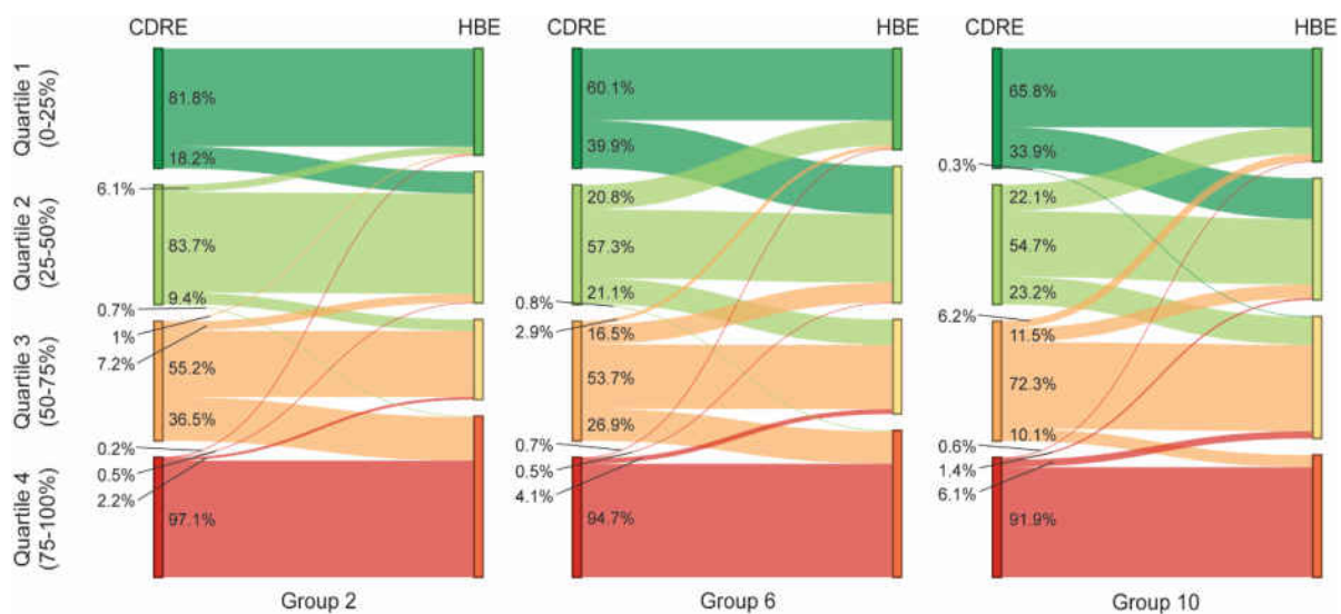
Figure B-3. The directions of potential SO 2 exposure misclassifications when the home-based exposure estimation method was used and when CMAQ fields were used.
