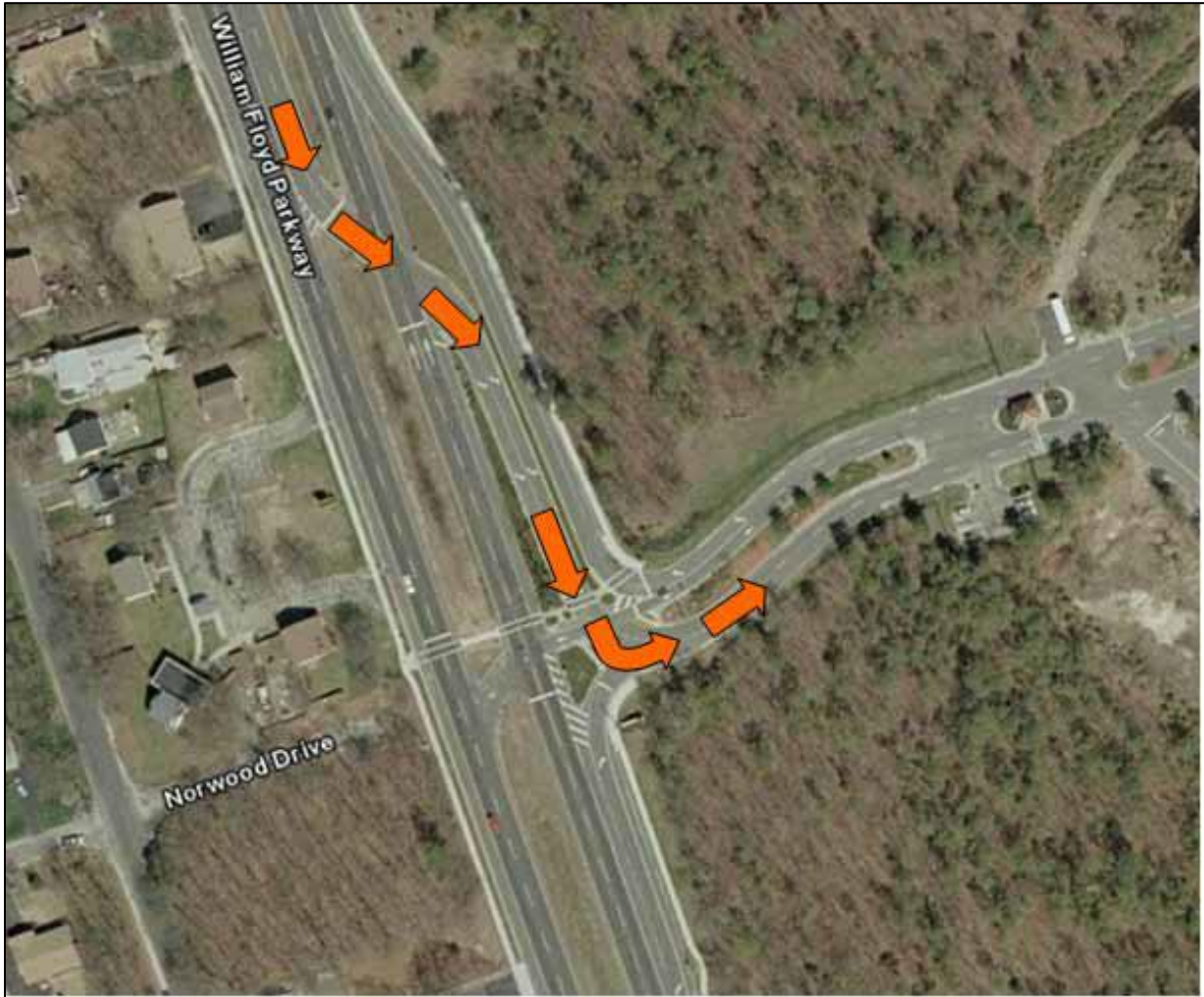
Figure 2: Left-turn crossover movement at a three-legged partial DLT in Shirley, New York
