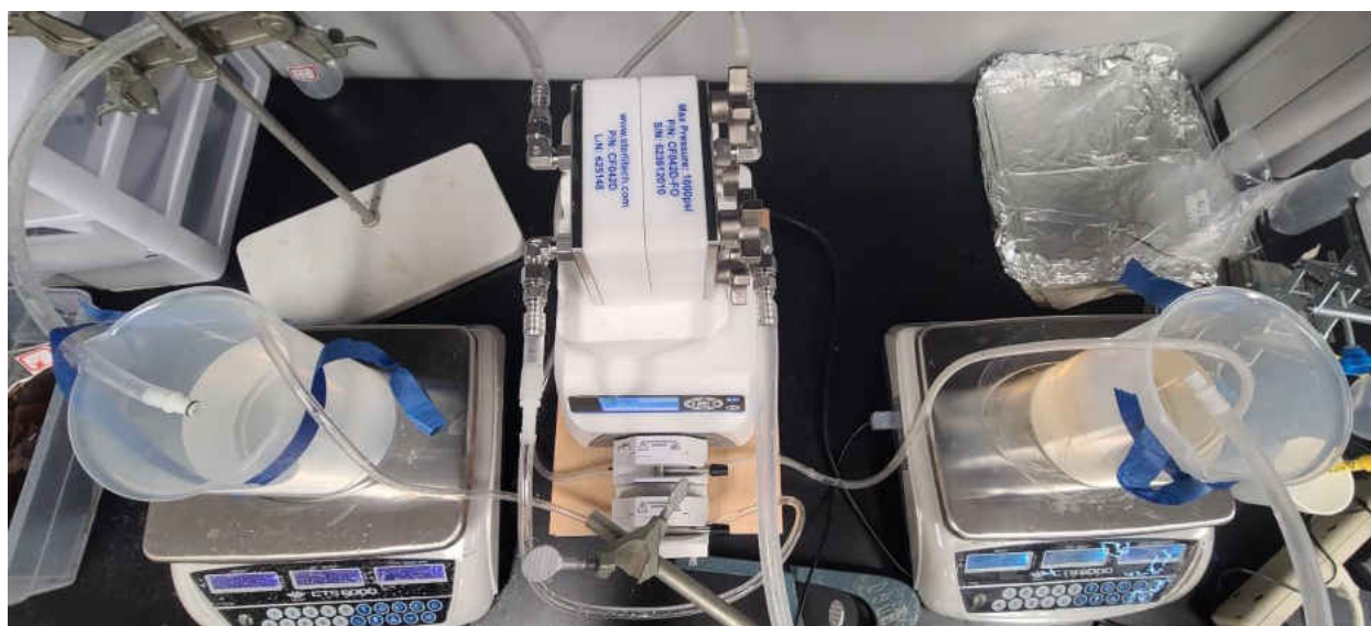
Figure 4. Bench-scale forward osmosis setup.
