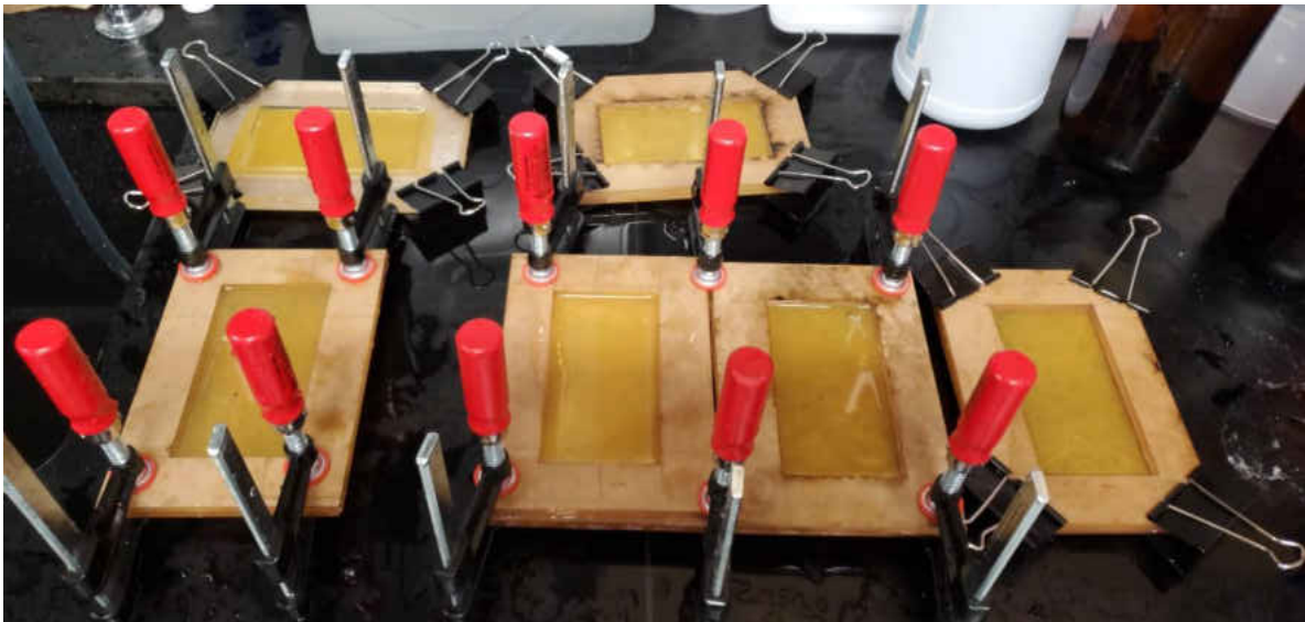
Figure 3. Customized dip coating setup for applying polyelectrolyte layers on the membrane.
