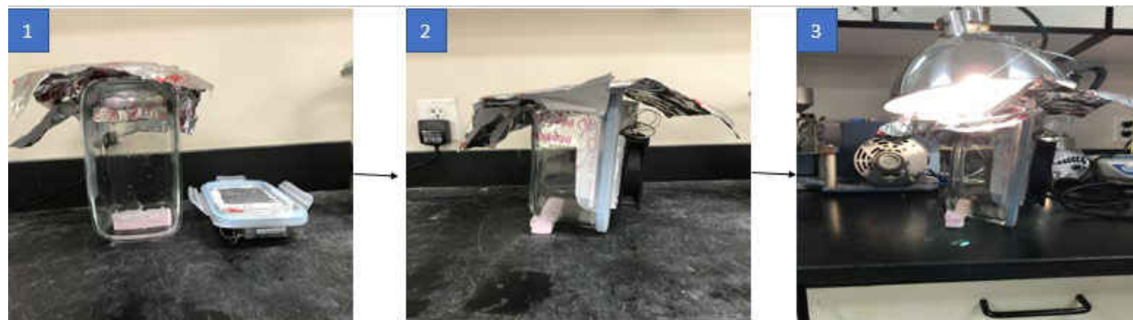
Figure 21. Deswelling test and sunlight simulation.
