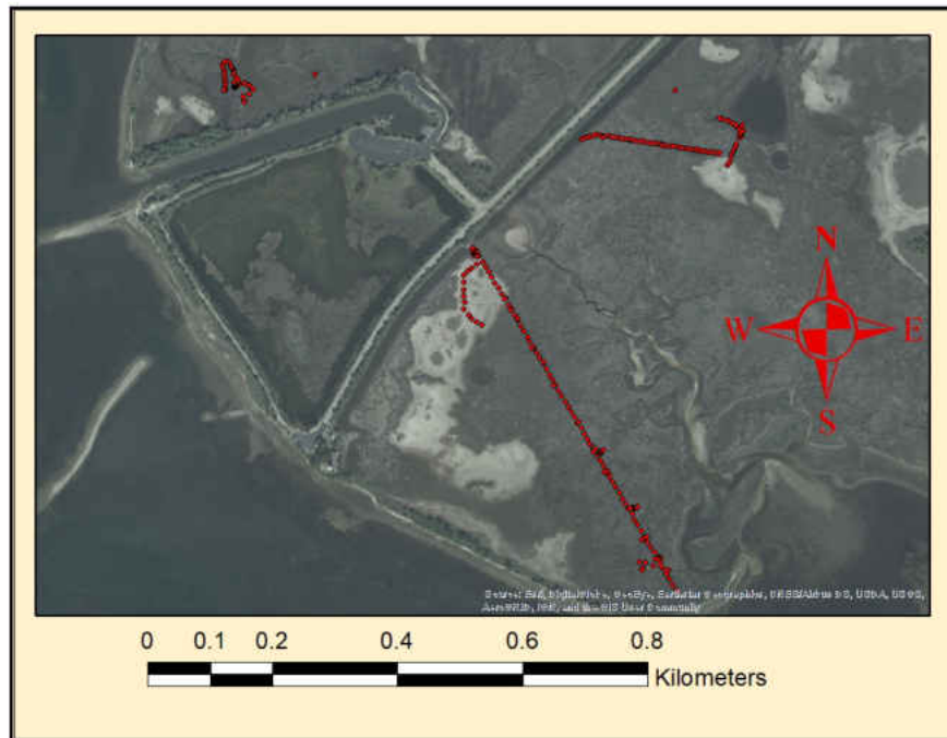
Figure 2. RTK survey conducted in the study area during two field visits (Summer 2017 and Spring 2018)
