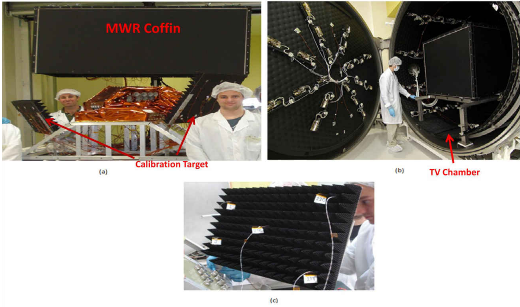
Figure 4-16 TV calibration test. a) MWR instrument with blackbody target and MWR coffin (aluminum box), b) MWR coffin inside TV chamber, c) blackbody target with the five temperature sensors.
