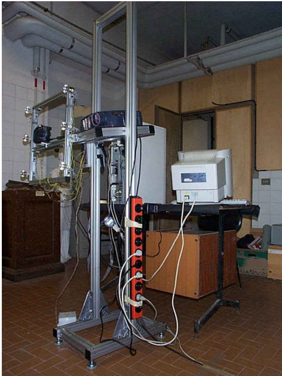
Figure 2.1: A low cost structured light 3D scanner [70].
