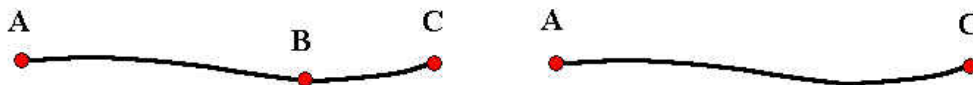
Figure 4.2: An example of a triplet collinear test of corner B between three consecutive corners A , B , and C : the initial corners (left) and the corners after the triplet collinear test (right).
