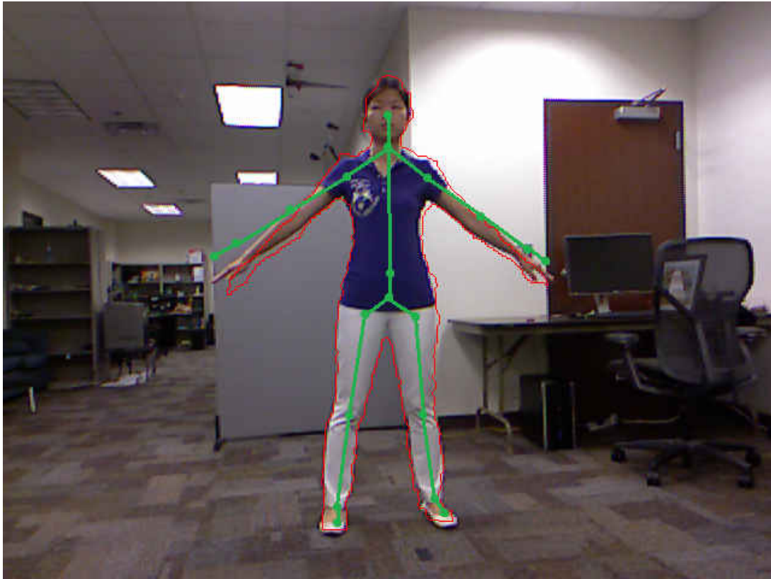
Figure 6.5: Latency between different Kinect data: (Background) the color image; (Red) the outline of the participant's tracking result; (Green) the saved skeleton information.
