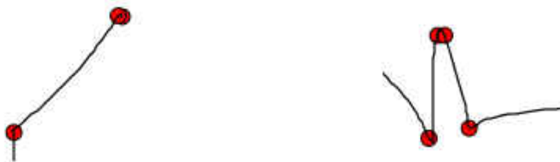
Figure 4.6: Two examples of sharp noise: caused by a hook (left) and caused by a sharp angle (right).
