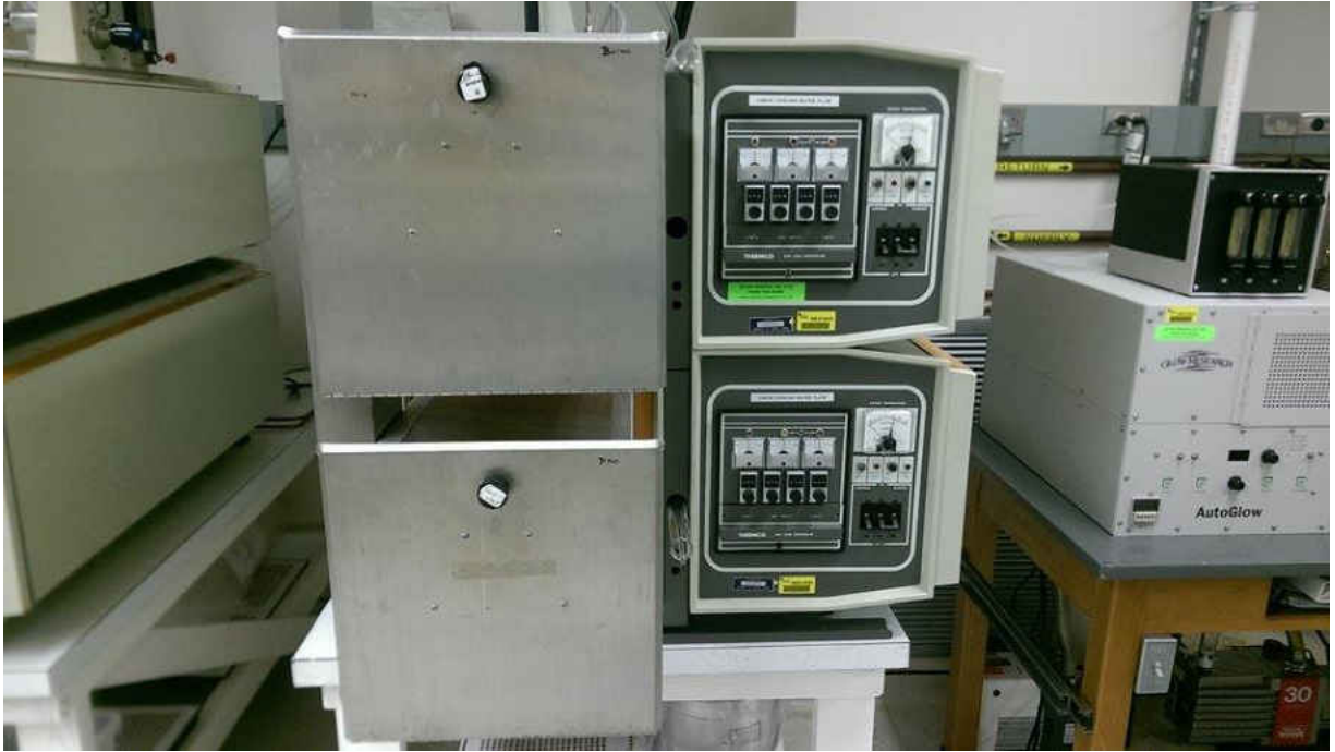
Figure A.1: Oxidation and Diffusion Furnaces
