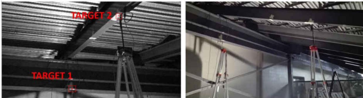
Figure 50 Two structural members monitored for human comfort
