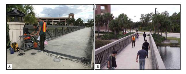
Figure 42 A: A perspective view from the footbridge and the data collection setup; B: The footbridge under the uncoordinated walking excitation of a group
