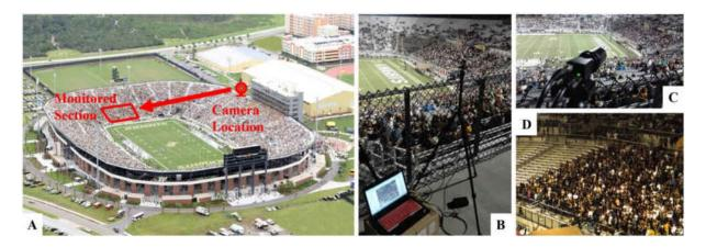
Figure 18 A: Overlook of the stadium showing the monitored section and the location of the camera; B: Experiment setup; C: The computer controlled industrial camera; D: One sample frame from the camera record
