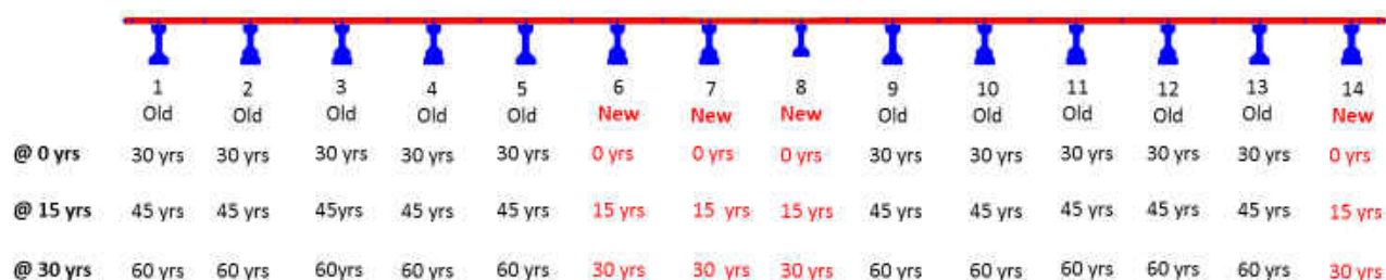
Figure 56: Aging Progression Schematics of Widened Bridge Members
