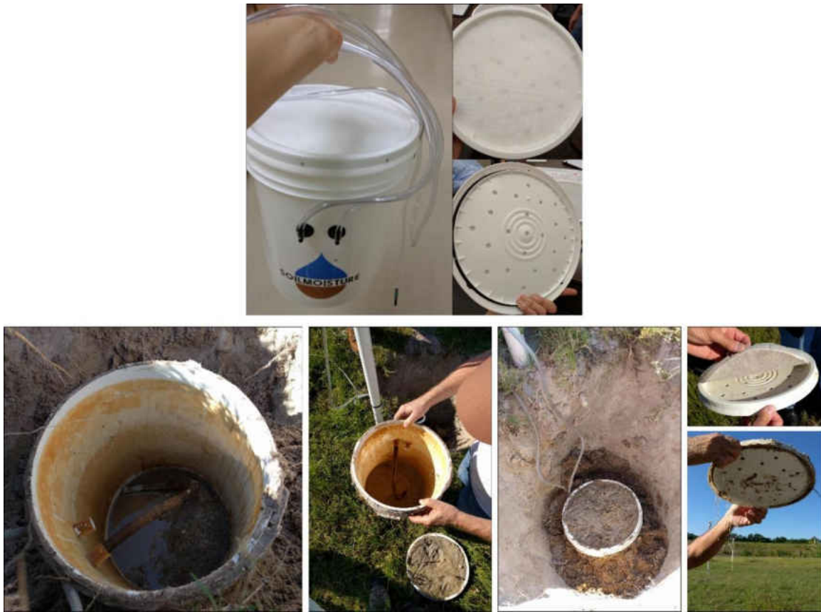
Figure 17. Lysimeter Prior to Installation and In-field.
