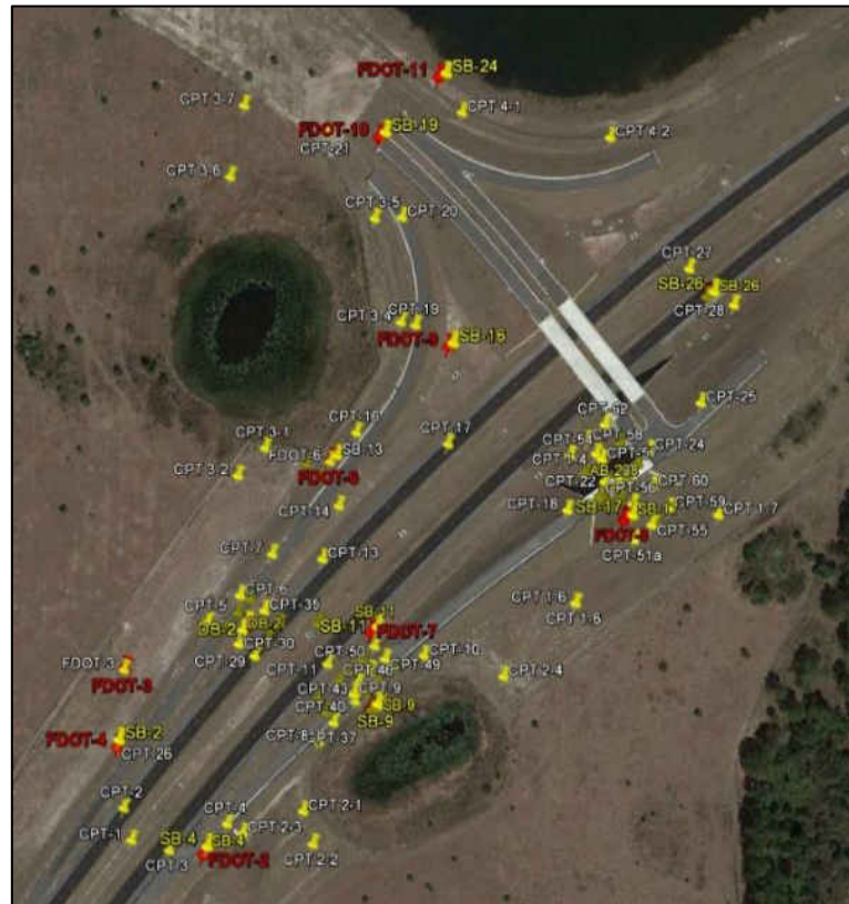
Figure 3-9: Layout of CPTs for Wekiva SR 46 connector project
