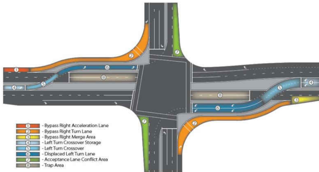
Figure 5 Layout of 2-Leg Continuous Flow Intersection (CFI) (UDOT CFI Guidelines, 2013)
