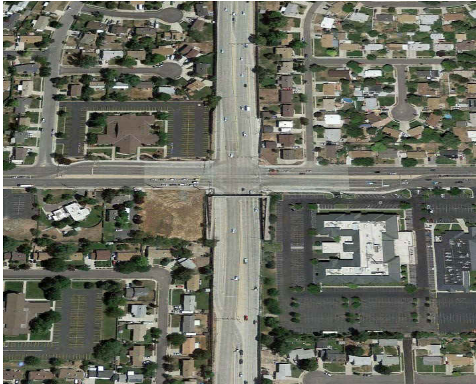
Figure 45 the Continuous Flow Intersection (CFI) at Bangerter Hwy and 4100 D. Rd, Utah, (Google Earth, 2016)
