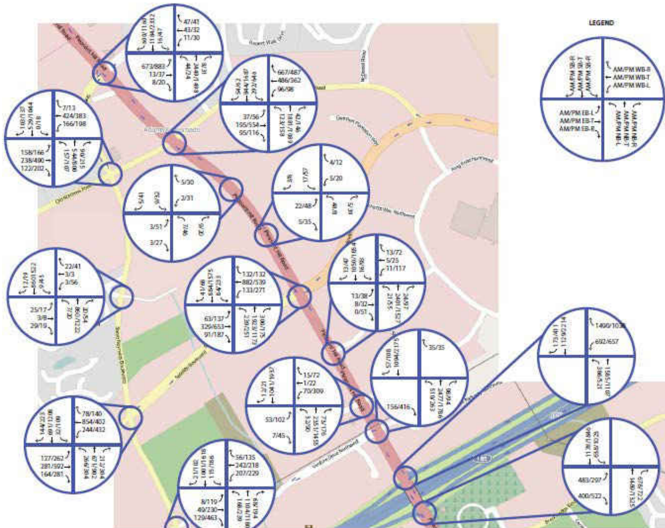
Figure 20 A Sample of Turning Movement Counts Summary and Their Locations for the DDI at Pleasant Hill Rd & I-85, Atlanta, GA (AM/PM), (FHWA- Reduced Data, 2015)
