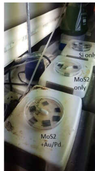
Figure 1. Absorbance of XTT-formazan at 470 nm as a method to monitor the production of ROS from MoS 2 , Au/Pd modified MoS 2 nanofilms and a substrate only (silicon wafer without MoS 2 as a control). The surface area of each nanofilms was identical with 3 cm 2 . 40 mL of XTT (0.4 mM) dissolved in phosphate buffered saline was used to submerge the samples while being exposed to 16,000 lx continuous cool-white fluorescent light illumination. Before tests, it was confirmed that there is no ROS production under dark condition using XTT.
