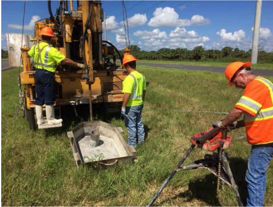
Figure A6: Sample Collection from SPT Test
