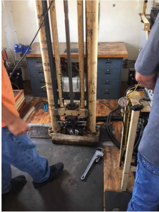
Figure A3: Cone Penetration Test Hydraulic Press for Ground Penetration
