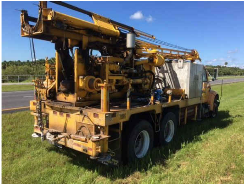
Figure A5: SPT Drill Rig on SR 415
