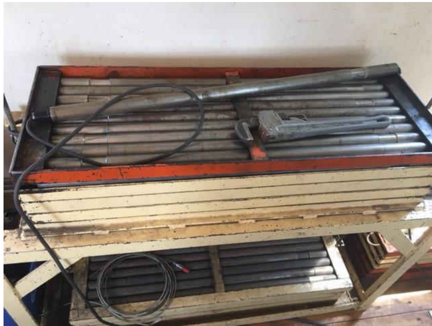
Figure A2: Cone Penetration Test Push Rods
