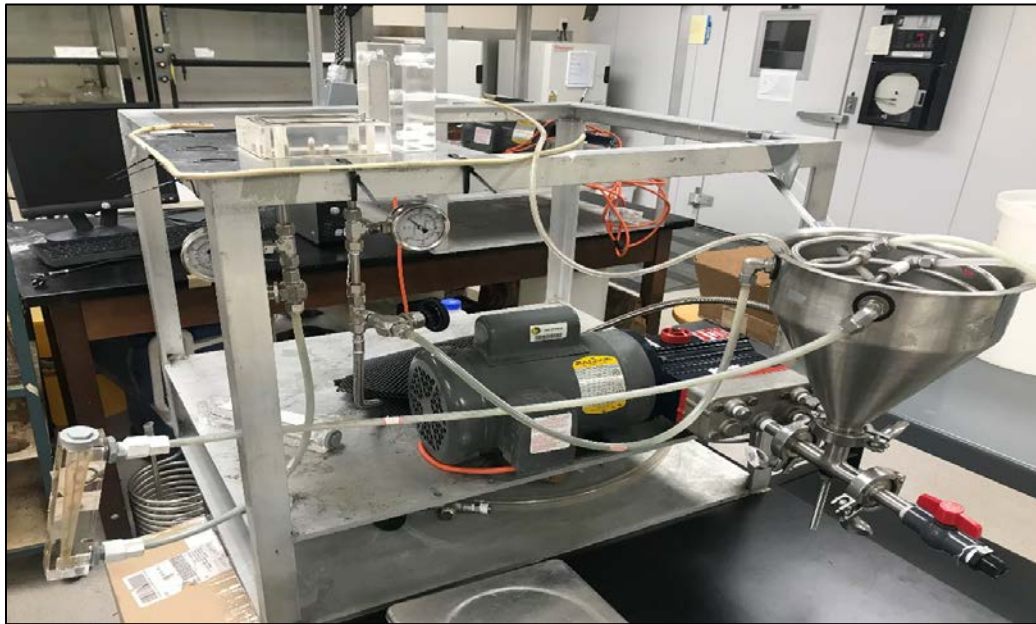
Figure 4-1: CF042 flat sheet testing unit
