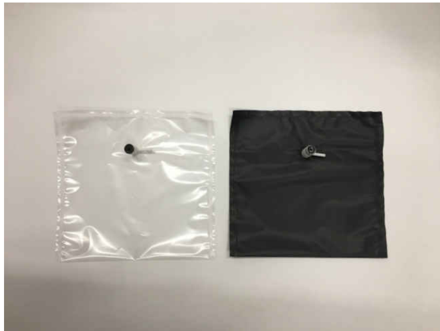
Figure 3-1: Empty 2.0 Liter Tedlar Bags Used for Photolysis Testing (left: clear test bag, right: black control bag)
