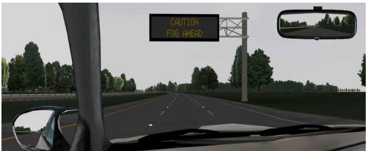
Figure 6: DMS Model with Caution Message
