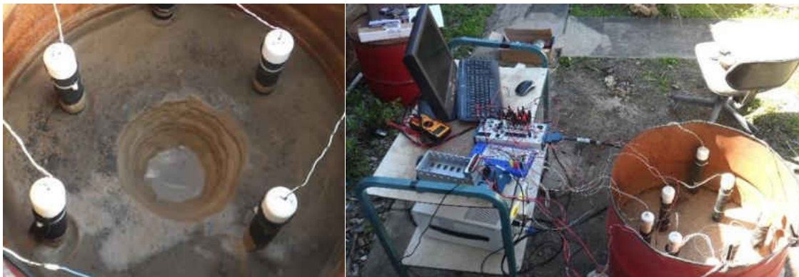
Figure 14: Sinkhole Physical Model Test Setup and sinkhole collapse.
