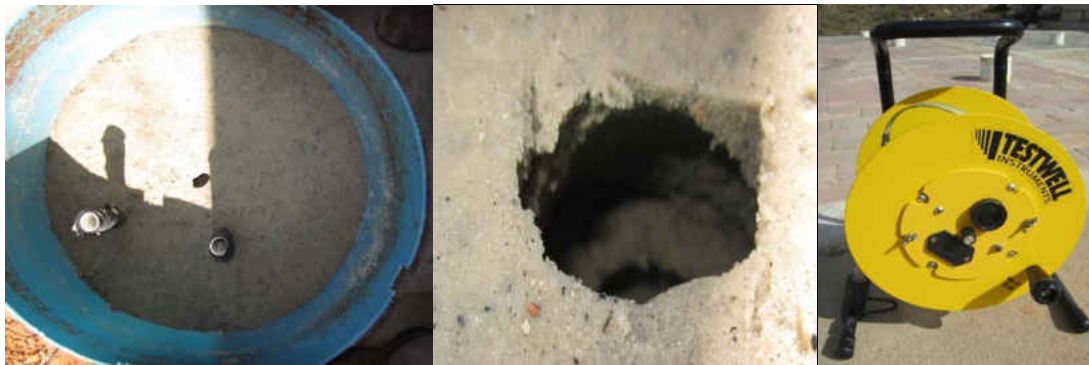
Figure 7: Second series of the initial tests and the Testwell water level meter
