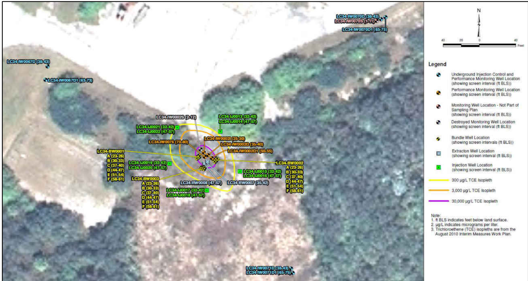
Figure 8: Recirculation Extraction, Recirculation Injection, and Monitoring Well Locations (NASA 2013)
