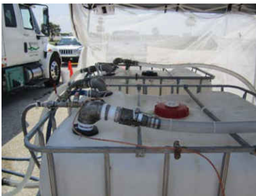
Bonding locations on mixing totes
