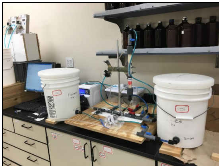
Figure A-6: Photo of the bench-scale hollow fiber membrane apparatus
