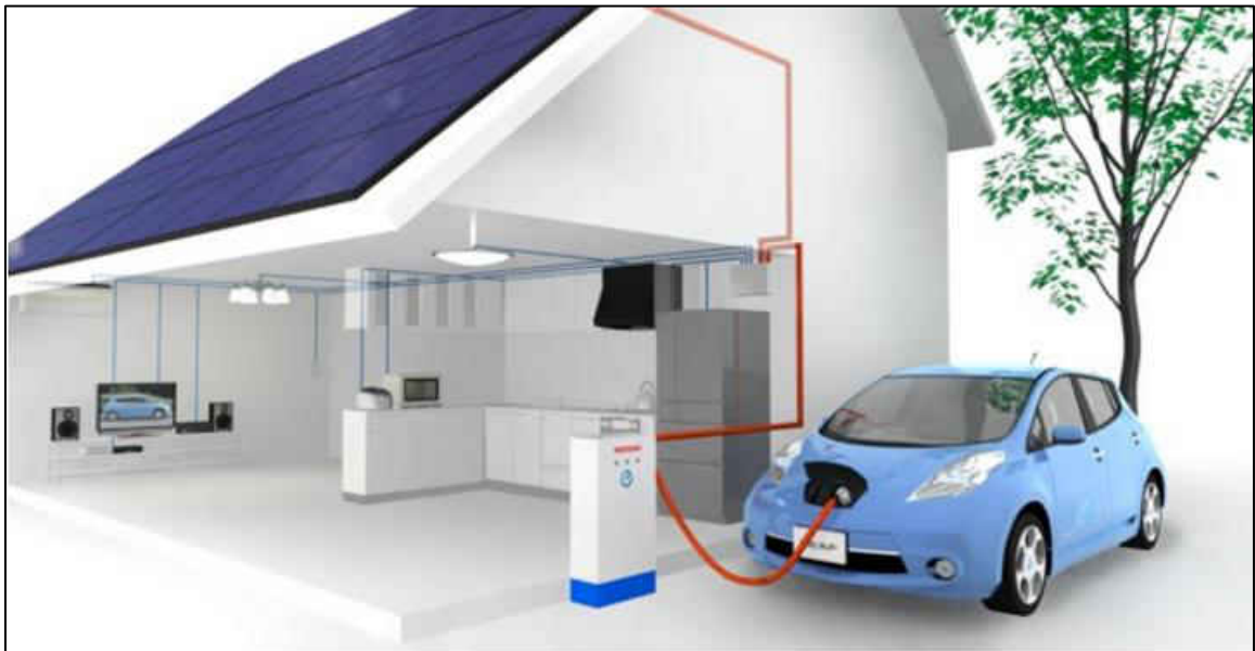
Figure 7. Power transmission from EV to building [72]
