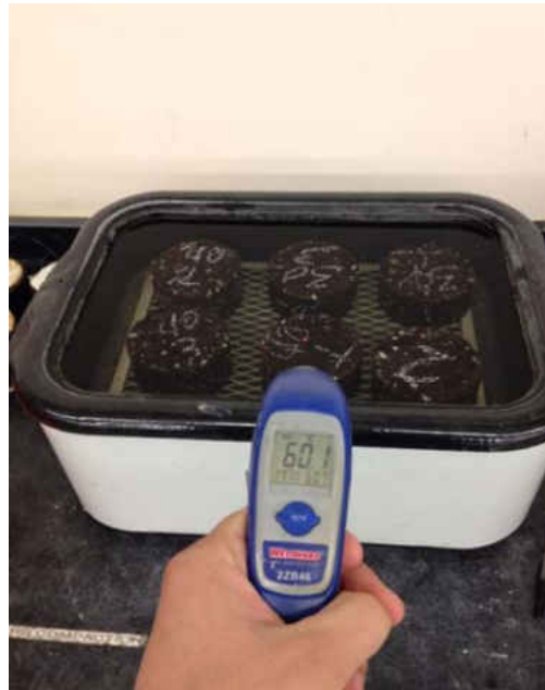
Figure 3-8. Wet subsets, soaking in distilled water at 60 °C for 24 hours
