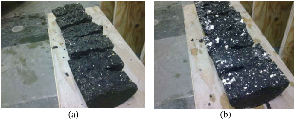
Figure 2-5. Fractured surface of specimens used in IDT tests: (a) 3.77% binder and 6% shingle (dry) and (b) 4.77% binder and 6% shingle (dry).
