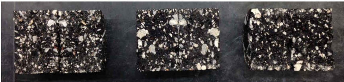
Figure 4-7: Photograph of the fractured surface for HMA 'V100A5.1'
