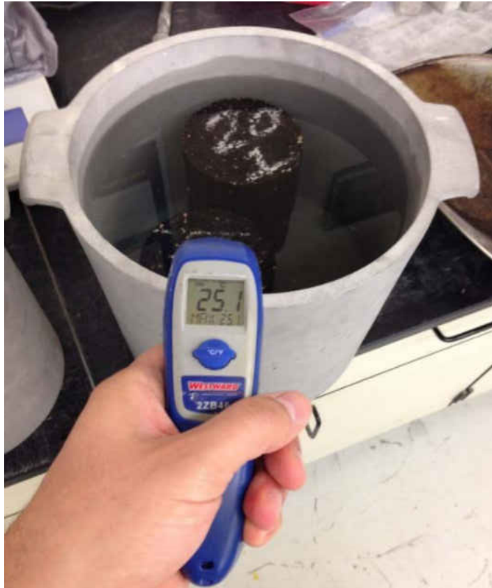
Figure 3-9. Wet subsets, adjusting the temperature by soaking in a water bath at 25 °C
