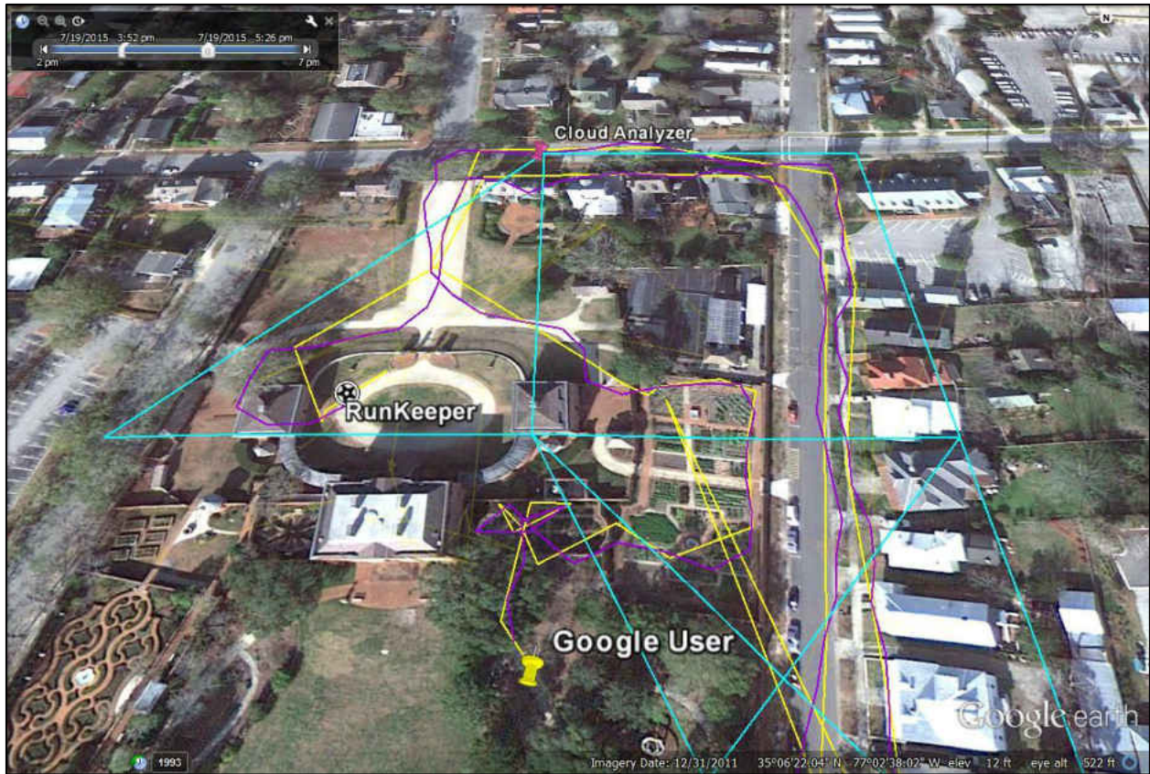
Figure 28 - Comparison of cached coordinates for same timeframe from RunKeeper (purple), Google user location history (yellow), and Cloud Analyzer (cyan)
