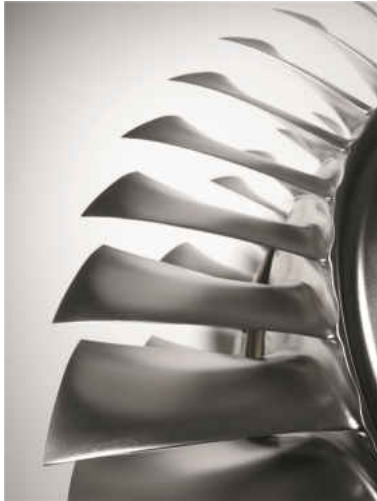
(a) Compressor blisk manufactured by GE (from [3])
