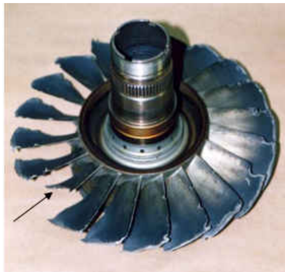
Figure 1.3: Failure of compressor blisk in Saab 340 aircraft with the fractured blade indicated (from [7])
